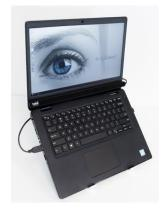
During a test, eye measurements and test responses are temporarily stored on an encrypted drive on the EyeDetect Station. When the EyeDetect Station is synchronized with the web server, all test and eye data are uploaded to the server for scoring.
